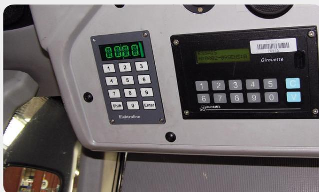
Using this code the vehicle pass automatically through all switches until its final destination.
