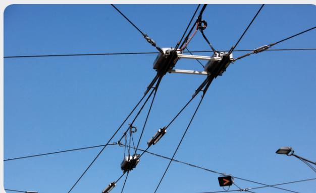
Switches are automatically set by VETRA system. Driver is only informed about actual status of the switch.
